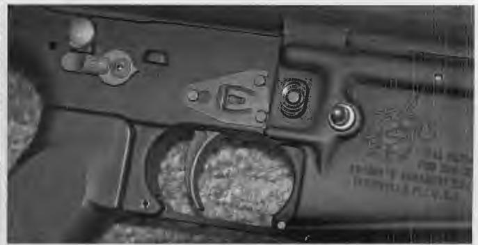
(left) This close-up illustrates the detail of the PDW's barrel machining and unique muzzle brake/flash suppressor. (right) Here the retainers for the PDW's fire control pins is seen. There are three pins instead of the M16's two.
