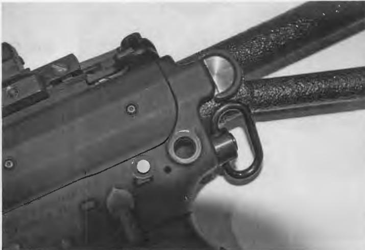
This close-up shows the PDW's folding stock mechanism and sling mounts.
