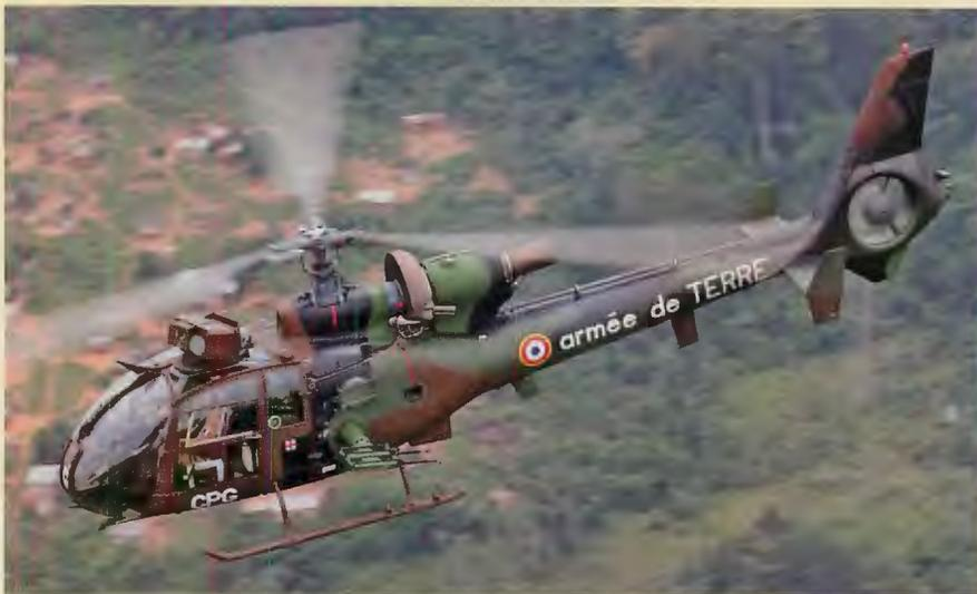
French troops are supported by the ALAT (Aiation Legere de l'Armee de Terre) Puma and Gazelle helicopters. The AT Gazelle shown here can mount the HOT missile, which are usually stored at the base. They are primarily used as an observation platform, with the all-weather/night VIVIANE camera, mounted here on the cockpit roof.
