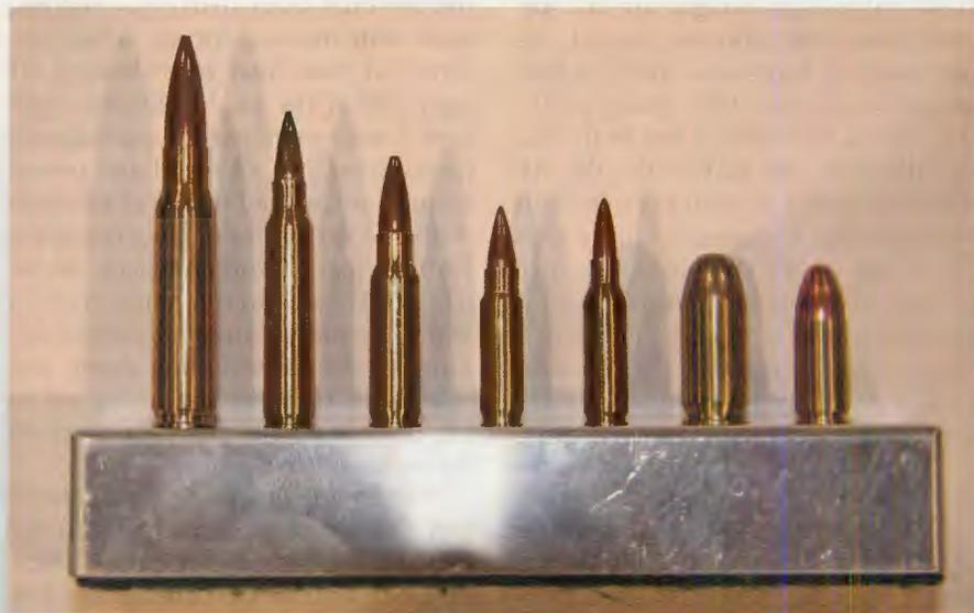
Here a cartridge comparison includes (from right to left) the 9x19mm, .45 ACP, 4.3mm H&K/PDW, 5.7mm FN/PDW, 6x35mm KAC/PDW, 5.56x45mm and 7.62x51mm rounds.
